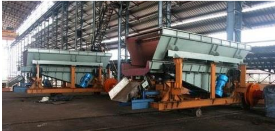
Figure 2.1.4a: Vibrating feeder for induction furnace
