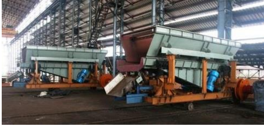
Figure 2.1.4a: Vibrating feeder for induction furnace
