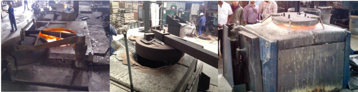
Figure 2.1.3: Different options for lid mechanism for induction furnace
