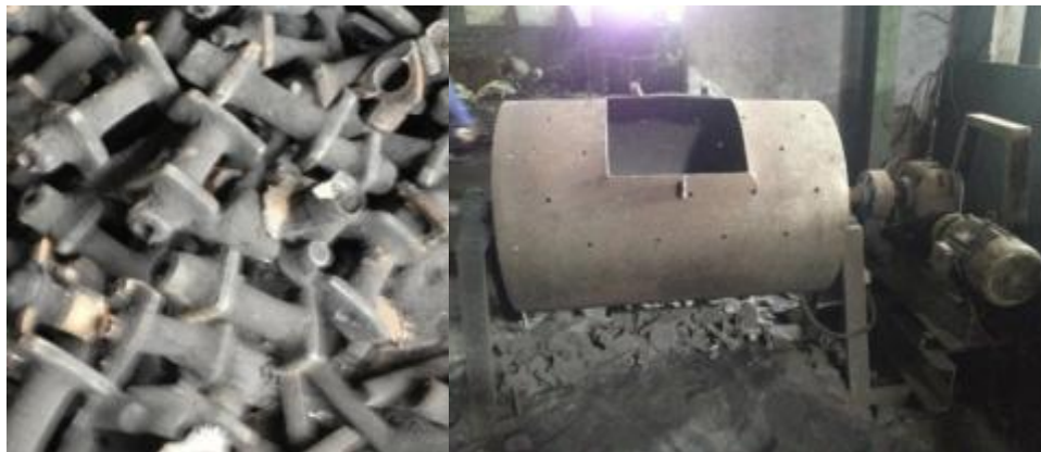
Figure 2.1.4b: Tum blast for runner and risers
