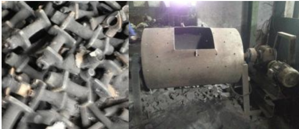
Figure 2.1.4b: Tum blast for runner and risers
