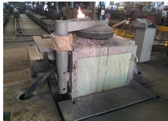
Lid mechanism for induction furnace crucible
