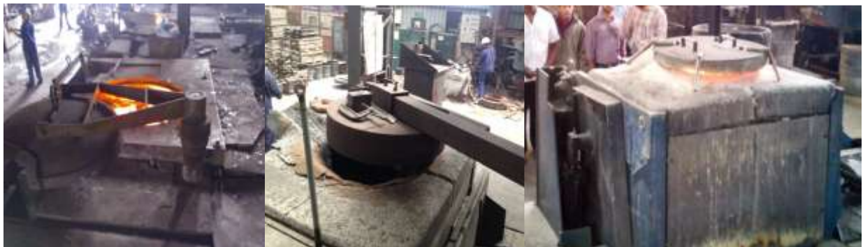
Different options for lid mechanism for induction furnace
