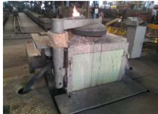
Lid mechanism for induction furnace crucible
