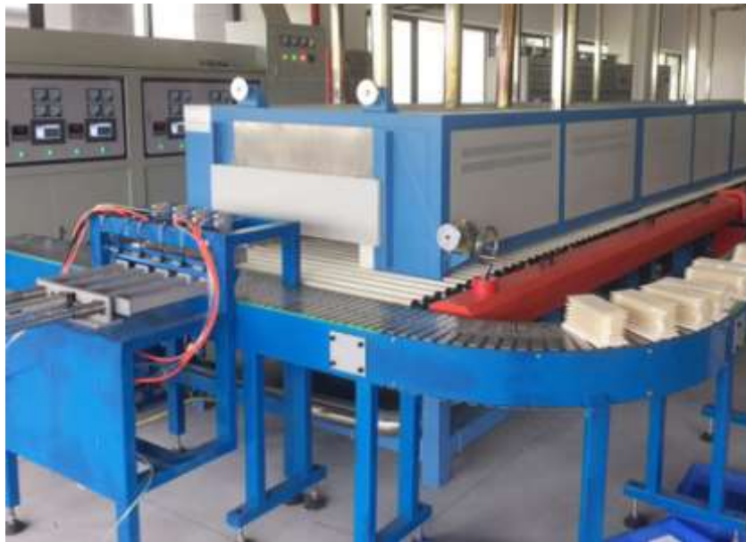
Roller hearth furnace
