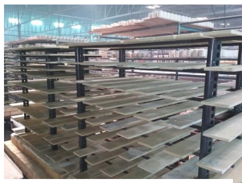
Low thermal mass (silicon carbide) kiln furniture
