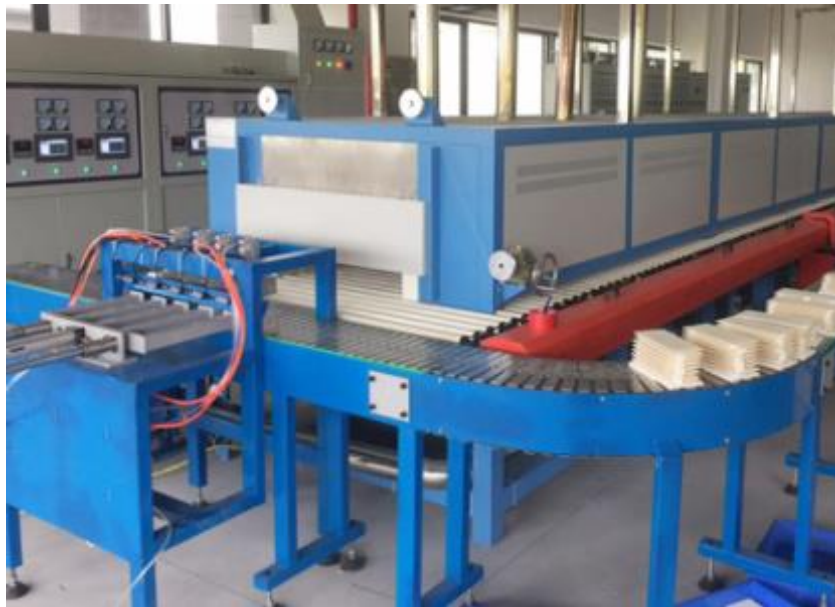
Roller hearth furnace
