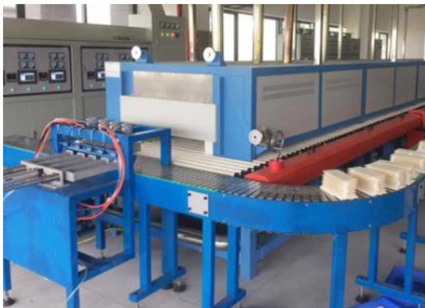
Roller hearth furnace
