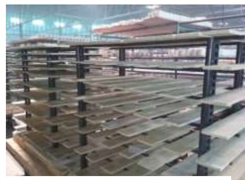
Low thermal mass (silicon carbide) kiln furniture
