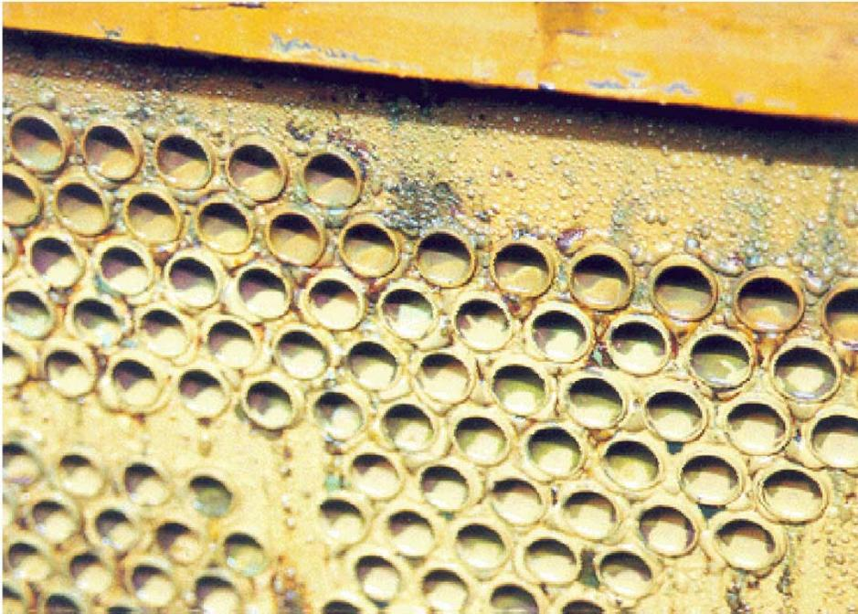
Tube before installation of Auto ball cleaning system
